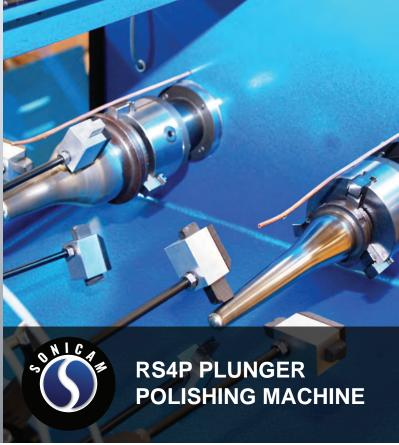
**Sonicam RS4P** provides a mirror finish surface on both new and repaired glass plungers for an efficient container glass production.
