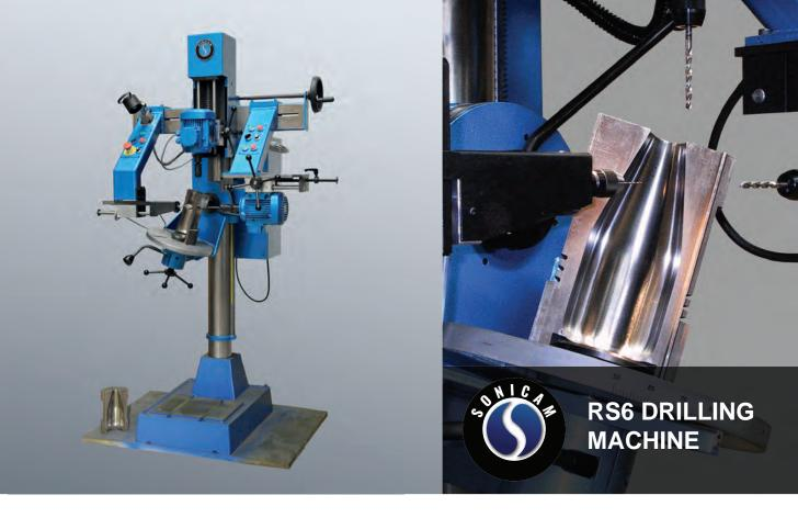
**Sonicam RS6** is drilling tiny vacuum channels inside the moulds.
