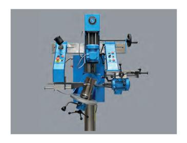
The mould cavity is fixed on a 360° swivel table for a better positioning.
